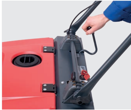
Lever for raising/lowering side brush
